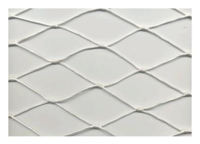
Regular 3mm PE netting with a breaking force of 140kg or 308 lbs
